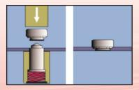
Installation of the Strux® Clinch Nut is essentially the same as the Strux® Clinch Stud. The retaining ring passes through the hole and as the displacement lobes seat, the engagement material flows into the retaining grove. However, the nut is supported by a spring loaded finder to ensure proper nut set. As the nut is staked, the finder retracts.
