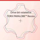
TORX PARALOBE™ Drive System has greater cross-sectional area versus TORX® and TORX PLUS® Drive Systems
